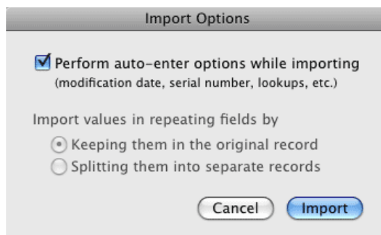
Figure 10.2: Second dialog to specify the options for importing. The checkbox should always be checked so that these auto-entered features are used.
